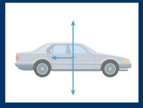
A free-body diagram shows only the forces acting on the object of interest—in this case, the car.
