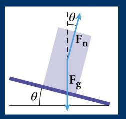
In the absence of other forces, the normal force is equal and opposite to the component of gravitational force that is perpendicular to the contact surface.
