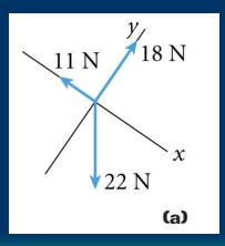
**Tip:** To simplify the problem, always choose the coordinate system in which as many forces as possible lie on the x- and y-axes.
