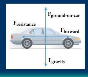
Although several forces are acting on this car, the vector sum of the forces is zero. Thus, the net force is zero, and the car moves at a constant velocity.
