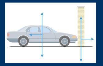
In a force diagram, vector arrows represent all the forces acting in a situation.
